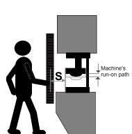
Fig. 35/2: Safety clearance and run-on distance
