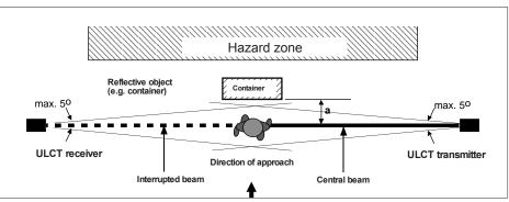
Fig. 14/1: Clearance to reflective surfaces
