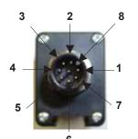
Pin 1 / white: Start Enabling of start with restart interlock, max. 24V DC +- 20%
