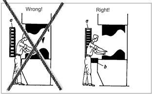
Fig. 15/3: Two cascaded safety light curtains to prevent infiltration from the rear
