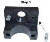
Insert 2 each of the accompanying adjustment screws via the through-bores into the M3 nuts pressed in at the rear.
