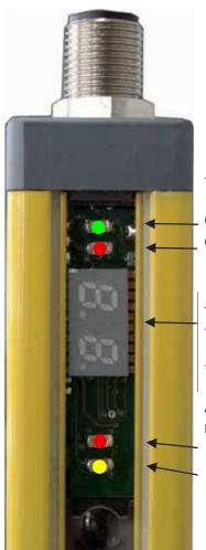
The LEDs and display on the receiver indicate the current operating status.
