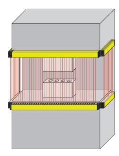
Safeguarding of a C-press on 3 sides without any obstruction by vertical deflecting mirrors.
