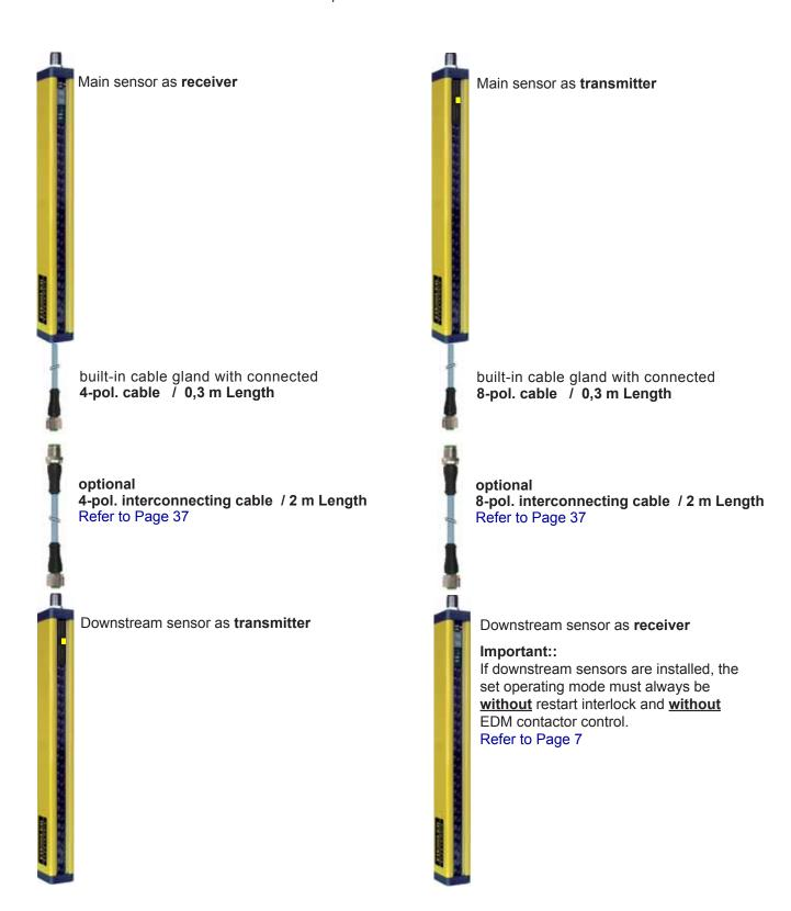
When 3 light grids are cascaded, the connection between the first and second downstream sensors is identical to that between the main sensor and first downstream sensor.
