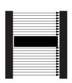
Fig. 25.1: Fixed or floating blanking with complete coverage of the light curtain's blanked section..
