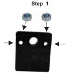
Press 2 M3 nuts each into the top ends of the widening elements
