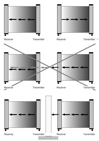
Fig. 16/3: Arrangement of two neighbouring light curtains
