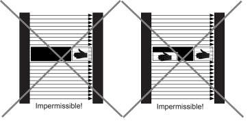
Fig. 25.2: Fixed or floating blanking with partial coverage of the light curtain's blanked section. Additional coverage is necessary.
