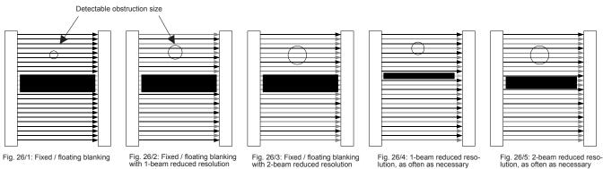
Fig. 26/2: Fixed / floating blanking with 1-beam reduced resolution Fig. 26/1: Fixed / floating blanking
