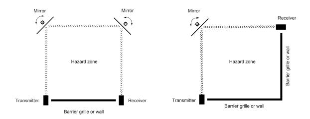
Reflection losses: Each time it is deflected by a mirror, the transmitted signal is attenuated. When using such mirrors, you should therefore account for the signal's maximum range and the number of required deflections. Make sure to mount transmitter, receiver and mirrors perpendicularly and check their alignment with a spirit level.
