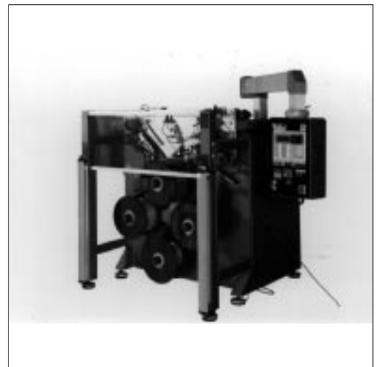
Guarding of a wiring harness assembler
