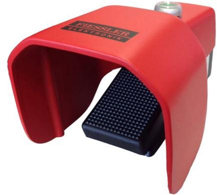
The foot pedal FE-FS1-SU1ASDO2V-U have 3 positions with a pressure point and a pedal lock with manual release, to control dangerous movements (for instance get down of a press brake ect...). It has 2 working contacts (1NO and 1NC) to drive the movement and one safety switches (2 positive opening NC contacts) to stop the movement.
