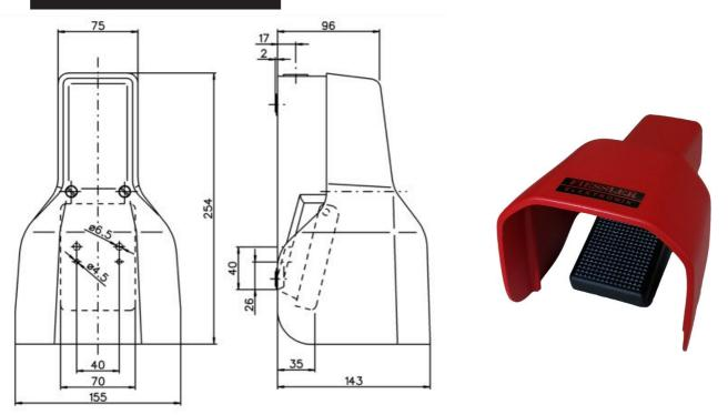
The foot pedal FE-FS1-SU1ASDO2-U have 3 positions with a pressure point to control dangerous movements (for instance get down of a press brake ect...). It has 2 working contacts (1NO and 1NC) to drive the movement and one safety switches (2 positive opening NC contacts) to stop the movement.
