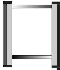
two-beam light grid with transmitter/receiver unit and mirror unit, range up to 10 m
