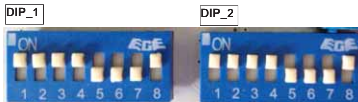
fig. 1 without permanent overrun measurement
